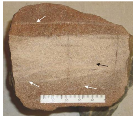
Figure 3. Photo of a boulder slab of the Penrith cataclastic rock in Coombs Wood, Vale of Eden. Single deformation band (white arrow) is approximate 1 mm width. The black arrow shows an example of small cataclastic zone. 5 cm scale on photo.
